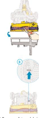
**B** Remove dirt or debris and check spindle is clean.
